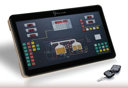
With up to 16 simultaneous touch points, the 15.6" Crystal Touch: TRUE Multi-Touch PCAP panel allows for increased functionality and multiple users to simultaneously benefit from the TRUE multi-touch interface. The combination of Atmel's maXTouch™ technology and Ocular's robust PCAP touch panel provides a sophisticated solution that can distinguish and disregard unintended touches while maximizing optical clarity, enhancing performance and creating an enjoyable user interface.
